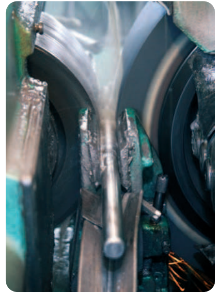
Pins are precision ground to enhance wear resistance and increase chain service life
