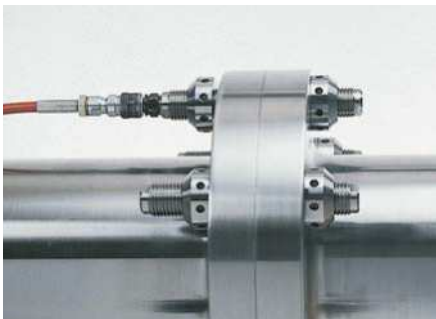
6. The pump is connected to the center of the bolt. Oil is injected to release the bolt from the sleeve. The bolt slides out of the taper and the sleeve immediately regains its original diameter.
