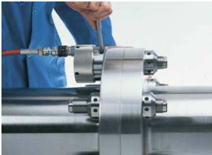
5. The tensioner is connected and pressurized and one nut is released.
