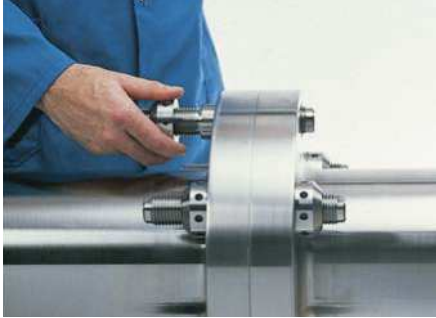
8. After unscrewing the nuts, the bolt and sleeve can be easily withdrawn by hand.
