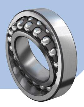
SKF self-aligning ball bearings have been solving problems with misalignment and shaft deflections for more than 100 years. This product has been redesigned continuously to the current optimized internal design featuring two rows of balls with a common sphered raceway in the outer ring.
