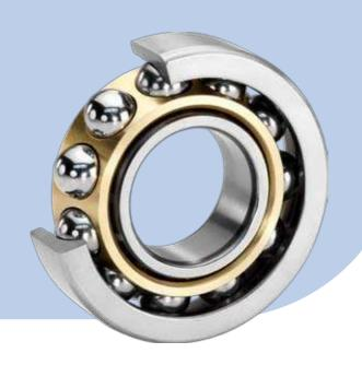
Designed to accommodate simultaneously acting radial and axial loads, SKF Explorer single row angular contact ball bearings incorporate features that enable these bearings to run cooler and smoother thereby reducing lubricant consumption and extending bearing service life by as much as 300 %.
